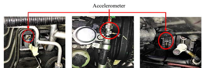
Fig. 6. Location of the sensors on (a) TVX, (b) AC pipe, and (c) compressor of the vehicle HVAC system.
