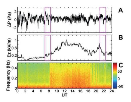
Fig. 1. Variations of atmospheric variables during the fog event of 3rd December 2001: A - atmospheric pressure (1s sampling), B - vertical electric field EZ (10s sampling), and C - spectrogram of atmospheric pressure variations. Rectangles show the intervals of fog formation and fog dissipation, respectively.
