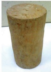
Fig. 5. A soil sample in the shape of a cylinder prepared for testing in a triaxial apparatus [34]
