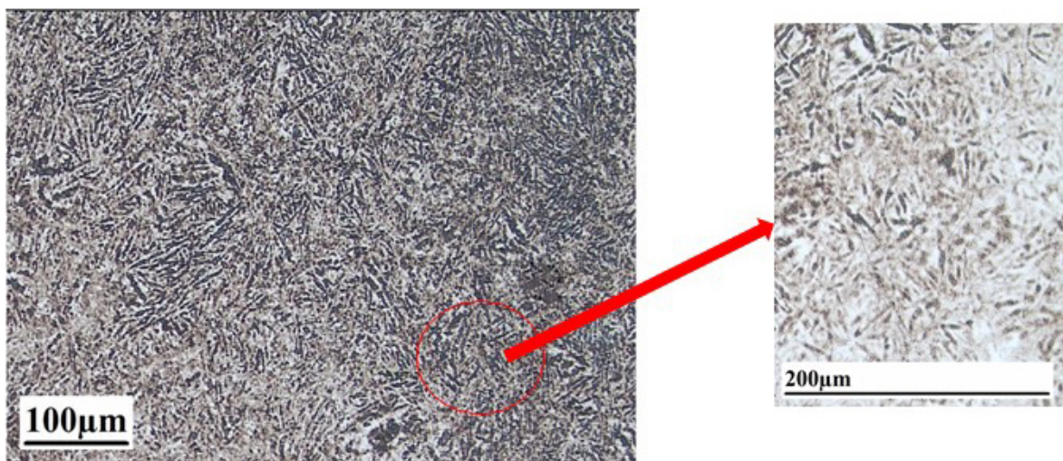
Fig. 3. Optical micrograph from the center of ER 80S weld metal
