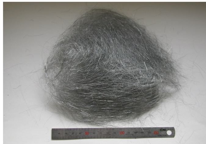
Fig. 1. A photograph of as-solidified Ti-7Zr-6Sn-3Mo (at%) fibers fabricated by a melt overflow process
