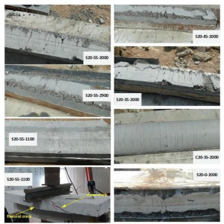
Fig. 6. Cracks in the test specimens.
