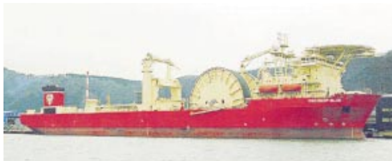
Fig. 2. Hyundai pipelay spread
