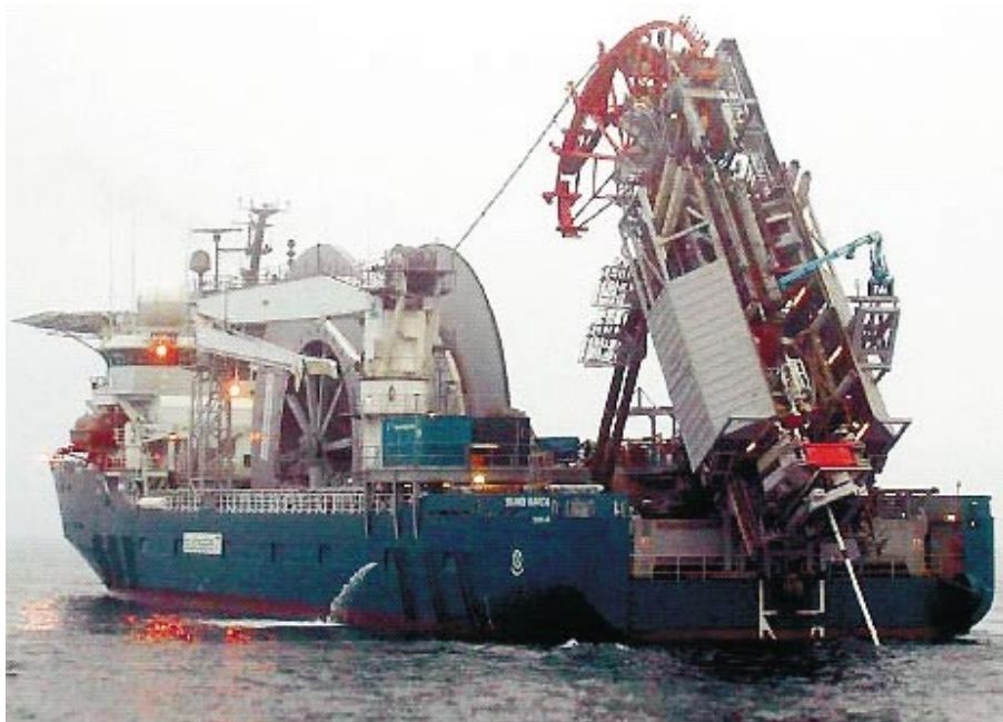
Fig. 4. Pipelay spread with a lay ramp and a tensioner
