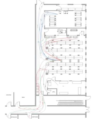
Fig. 9. Flow diagram for one order before changes, source: data provided by the enterprise.
