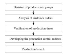
Fig. 2. The methodology of implementing production levelling in the analysed department; source: prepared by the author.
