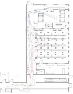
Fig. 10. Flow diagram for one order after changes, source: data provided by the enterprise.
