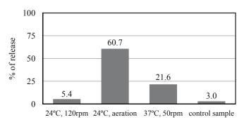
Fig. 4. Efficiency of indium release from ash sample A
