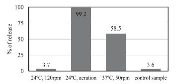
Fig. 1. Efficiency of rhodium release from ash sample A
