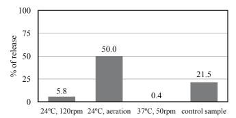
Fig. 5. Efficiency of chromium release from ash sample A
