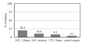
Fig. 6. Efficiency of rhodium release from ash sample B
