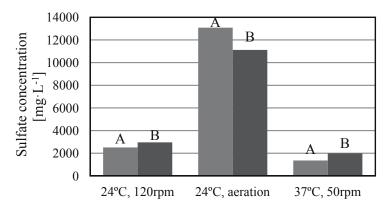
Fig. 9. Sulfate concentration in various variants of leaching culture after 5 days of bioleaching [mg·L-1]
