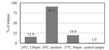
Fig. 2. Efficiency of cadmium release from ash sample A
