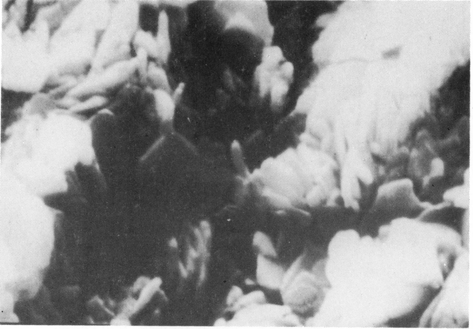
Fig. 25. Taranakite. Flaky structure of crystal aggregate, locally hexagonal habit is discernible. Scanning electron microscope image, magnification 9610 ×
