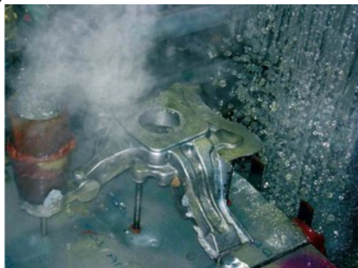
Fig. 1. The ablation casting process: a - the beginning of the ablation process, b - ready casting [8]
