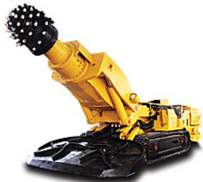
Fig. 2. Roadheaders equipped with: (a) transverse cutting heads (Famur, 2015) and (b) longitudinal cutting heads (Sanyhe, 2015)
