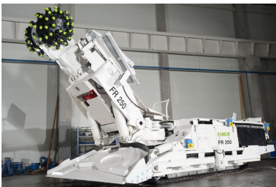
Fig. 2. Roadheaders equipped with: (a) transverse cutting heads (Famur, 2015) and (b) longitudinal cutting heads (Sanyhe, 2015)
