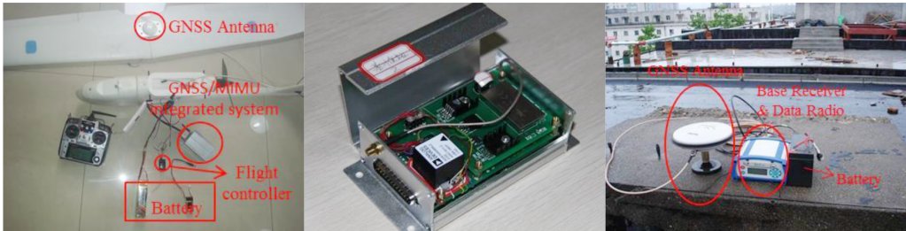
Fig. 3. The airborne equipment (left), GNSS/MEMS-INS prototype system (middle), and RTK base station (right).
