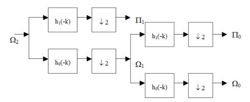
Fig. 2. Two decomposition levels of the DDWT ( $\Omega_2-$  the analyzed signal,  $\Pi_{1-0}-$  detail coefficients of the analyzed signal,  $\Omega_{1-0}-$  approximation coefficients of the analyzed signal.
