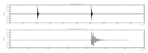
Fig. 8. The reconstruction of detected disturbances in simulated signal (Fig. 6.) (5 decomposition levels and wavelet db2).
