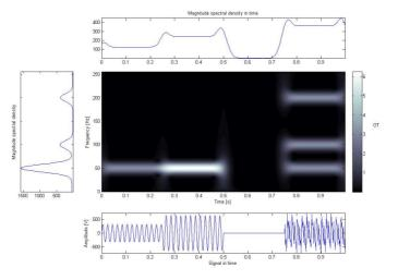
Fig. 9. GT time-frequency plane of signal 1.
