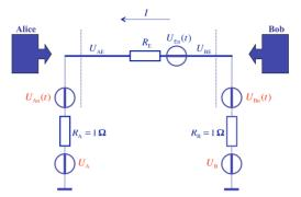
Fig. 5. An outline of the situation encompassing correct physics represented by non-zero Johnson noise voltages of the resistors. The impacts of  $U_{An}$  and  $U_{Bn}$  are significant: for GAA's absurdly limited Eve it provides non-perfect eavesdropping and a continuous change of the information leak when  $R_E$  converges to zero. Perfect eavesdropping can be achieved only after infinitely long time-averaging, which is unphysical.
