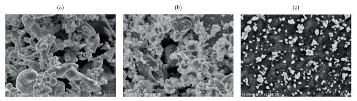
Fig. 1. SEM micrograph of received powders (a) aluminium, (b) silicon, and (c) zirconium carbide
