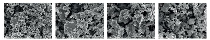
Fig. 2. SEM micrograph of the various wt. % of powder after mixing (a) Al-12Si, (b) Al-12Si-5ZrC, (C) Al-12Si-10ZrC, and (d) Al-12Si-15ZrC
