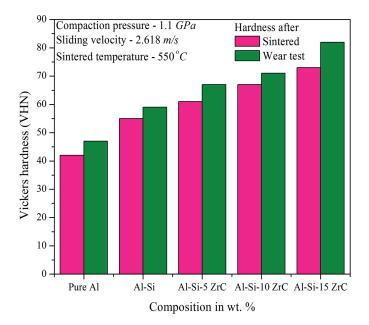
Fig. 5. Vickers hardness of composites at various wt. % of ZrC
