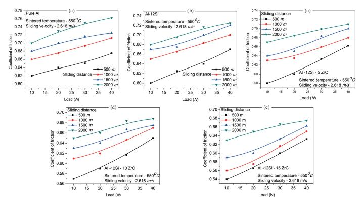
Fig. 6. Cofficient of friction as a function of load: (a) Al, (b) Al-12Si, (c) Al-12Si-5ZrC, (d) Al-12Si-10ZrC, and (e) Al-12Si-15ZrC
