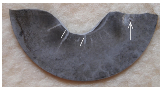
Fig. 5. The lower surface of the Pf insulator middle shed sample. The arrow points at the place where the shed was punctured. The lines denote the area in which the surface profile was examined. The measurement was taken from the left to the right hand side
