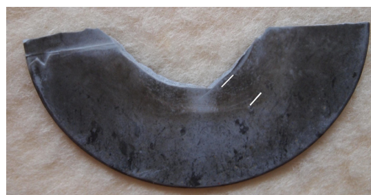
Fig. 9. The upper surface of the Lt insulator middle shed sample. The lines denote the area under examination with a bigger intensity of and small cracks in the dark coating. The measurement was taken towards the shed edge
