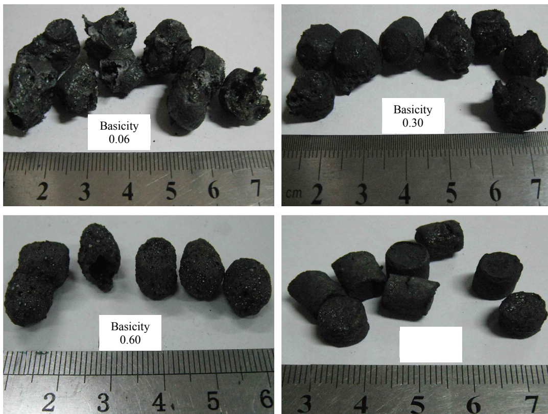
Fig. 6. Reduced briquettes after reduction roasting at the different basicity (briquettes with 12% coke fines roasting at 1250°C for 30 min)
