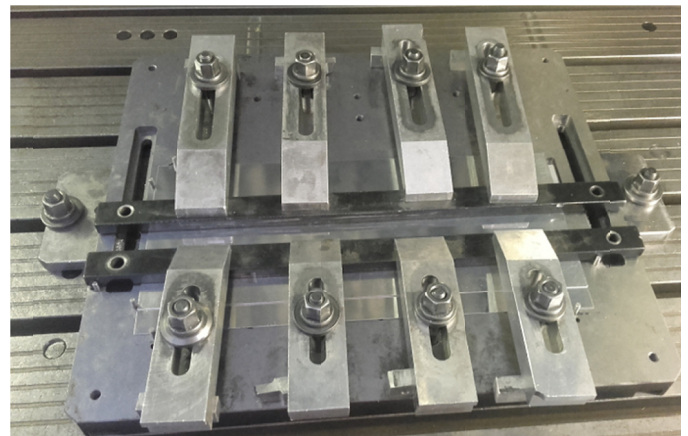
Fig. 2. The clamped aluminum sheets prepared for FSW process
