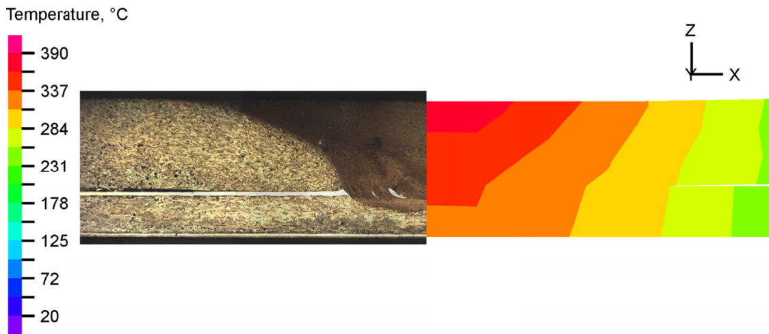
Fig. 9. Comparison of macrostructure and calculated temperature field in the joint cross-section
