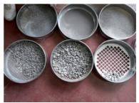
Fig. 1. Selection and screening of waste road concrete
