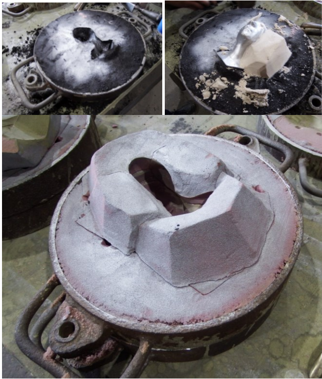
Fig. 1. Selected stages of moulding process: pattern batch, sand-piece, drag – lower part of mould [2]
