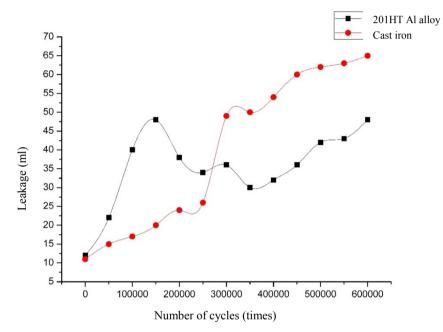
Fig. 2. Leakage curve of different material
