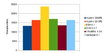
Fig. 2. Results of NIC throughput test.
