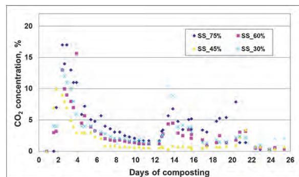
Fig. 7. CO<sub>2</sub> emission in gasses emitted from bioreactors; SS\_75%, SS\_60%, SS\_45%, SS\_30% as in Table 1; source: own study
