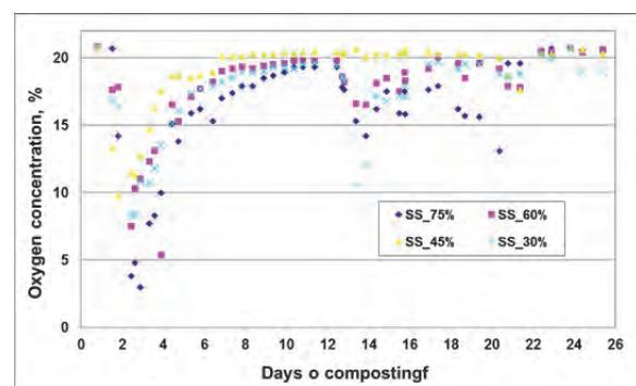
Fig. 4. Oxygen concentration in studied mixtures during composting process; SS\_75%, SS\_60%, SS\_45%, SS\_30% as in Table 1; source: own study
