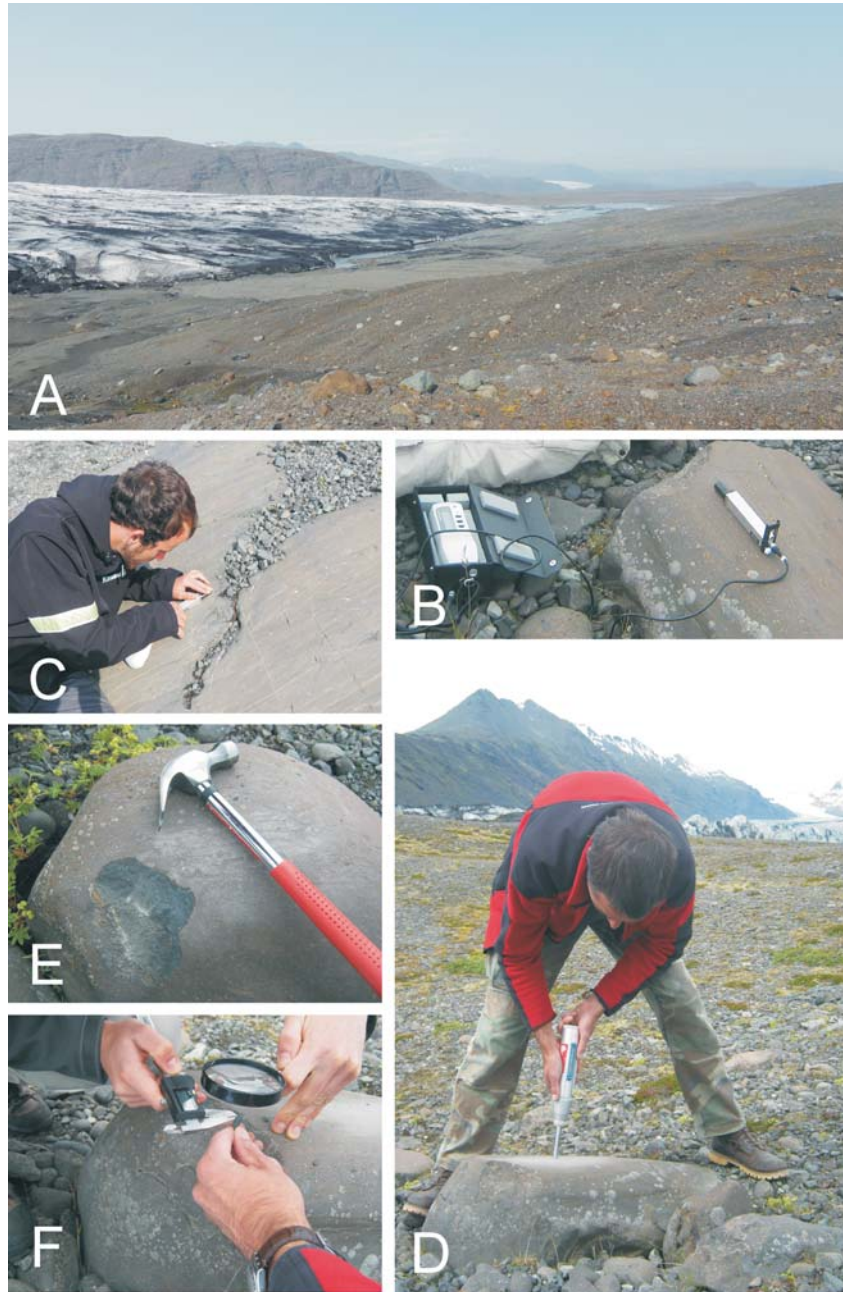
Fig. 2. General view on Skálafellsjökull marginal zone from SW corner towards NE (A); the Handysurf E35-B electronic profilometer (B); measurement of micro-roughness of glacially-abraded bedrock (C); obtaining Schmidt hammer rebound values from an abraded boulder (D); a boulder after chipping off a rock fragment for measuring weathering rind thickness (E), notice difference in colour between oxidised weathering rind and a fresh interior of rock; and measurement of the weathering rind thickness using a micrometer and a magnifying glass (F).
