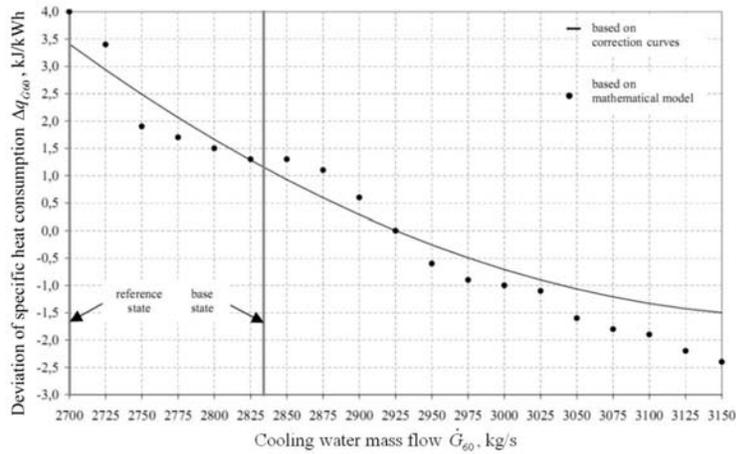
Figure 8. Deviation of specific heat consumption  $\Delta q_{T\dot{G}60} = q_{\dot{G}60} - q_{\dot{G}60}^b$  caused by deviation of cooling water mass flow from base state in turbine's condensing mode.
