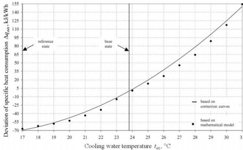
Figure 9. Deviation of specific heat consumption  $\Delta q_{Tt60} = q_{t60} - q_{t60}^b$  caused by deviation of cooling water temperature at the inlet of condenser from base state in turbine's condensing mode.
