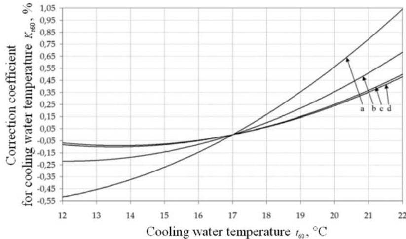
Figure 6. Correction curve of specific heat consumption in bleed-condensing turbine on cooling water temperature – condensing mode.
