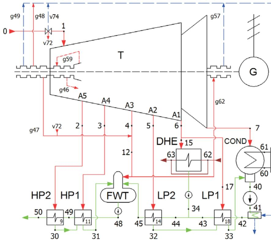
Figure 1. Diagram of the 70 MW<sub>el</sub> CHP unit with bleed-condensing turbine.
