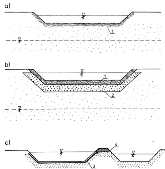
Fig. 9. Schemes of infiltration reservoirs: a) natural basin, b) filtration layer, c) infiltration reservoir with preliminary settling; 1 – soil, 2 – filtration layer, 3 – plastic sealing, 4 – overflow (pipeline)
