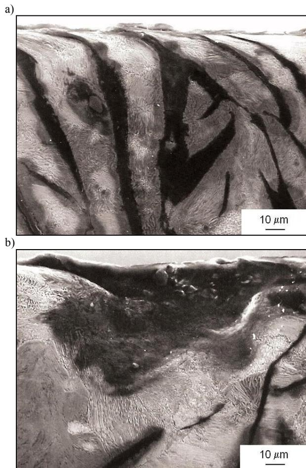
Fig. 3. A view of the cylinder liner bearing surface in the piston dead center region (a-b)
