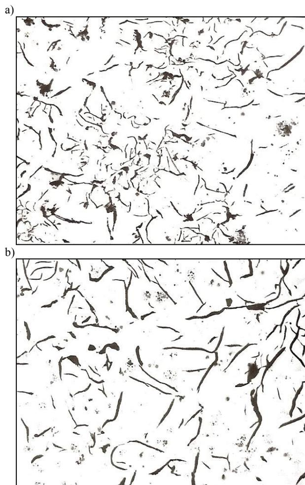
Fig. 4. Structure of the experimental liner casting: (a) in the area adjacent to the inner surface and (b) at half thickness of the casting wall. Non-etched section. Magnification 110×
