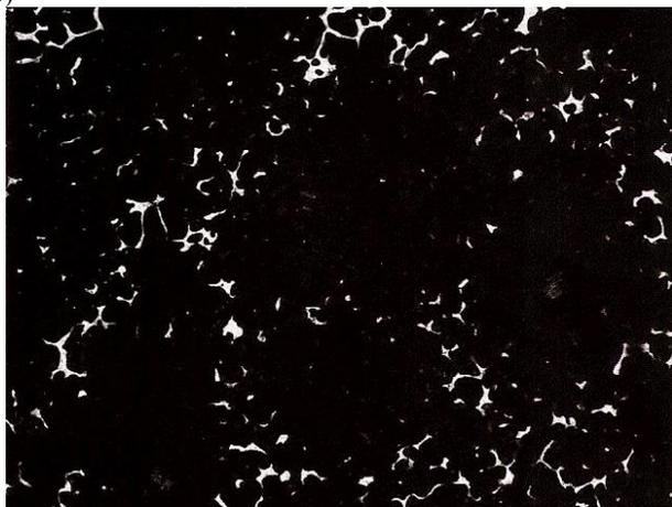
Fig. 6. Distribution of phosphide eutectic in the experimental liner casting: (a) in the area adjacent to the inner surface and (b) at half thickness of the casting wall. Etching in 4% HNO<sub>3</sub>. Magnification 50×.
