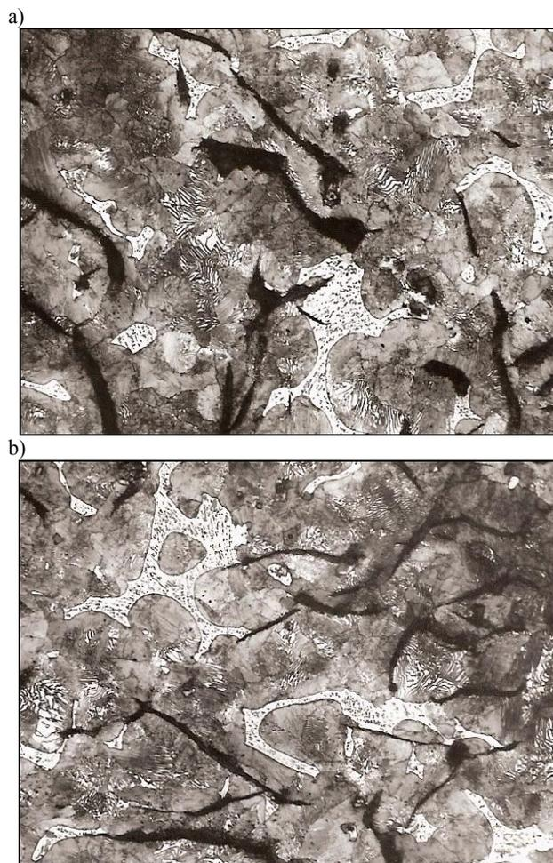
Fig. 5. Structure of the experimental liner casting: (a) in the area adjacent to the inner surface and (b) at half thickness of the casting wall. Etching in 4% HNO<sub>3</sub>. Magnification 250×
