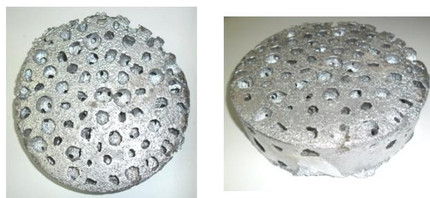
Fig. 9. Casting (AlSi10MgMn) – type II
