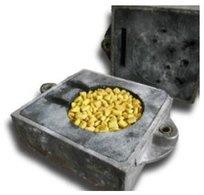
Fig. 3. Mold filled with precursors
