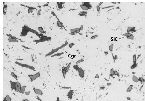
Fig. 1. Exemplary microstructure of AlMg10 + 8% SiC+2%  $\text{C}_{\text{gr}}$  composite, magn. 100 $\times$
