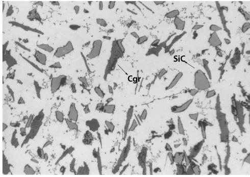
Fig. 2. Exemplary microstructure AlMg10 + 5% SiC + 5% Cgr composite, magn. 100×
