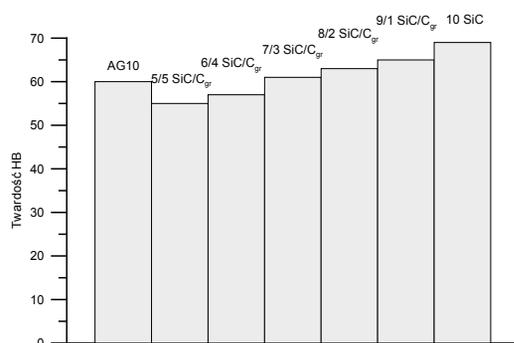
Fig. 8. Bar chart comparing hardness of examined materials
