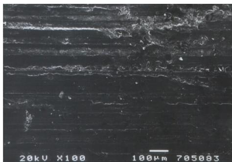
Fig. 7. Photomicrograph of sliding surface of the AlMg10 + (7% SiC and 3% C<sub>gr</sub>) composite, magn. 100×
