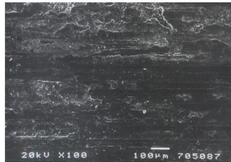
Fig. 6. Photomicrograph of sliding surface of the AlMg10 + (5% SiC and 5% C<sub>gr</sub>) composite, magn. 100×
