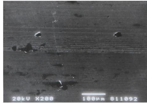
Fig. 5. Photomicrograph of sliding surface of the AlMg10 + (9% SiC and 1% C<sub>gr</sub>) composite, magn. 100×
