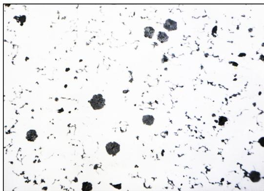
Fig. 4. Graphite precipitates in cast iron containing 3.77% Al (melt No. 6); non-etched microsection, magn. 100×
