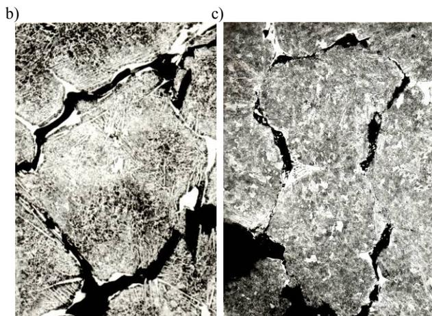
Fig. 2. Shrinkage macro- and micropores in the cracked mill roll of L180HMF cast steel; a) cracks along the boundaries of solidification grains, magn. 5 $\times$ ; b) cracks in the secondary cementite net, magn. 100 $\times$ ; c) cracks in the ledeburite net, magn. 60 $\times$ ; etched with Nital
