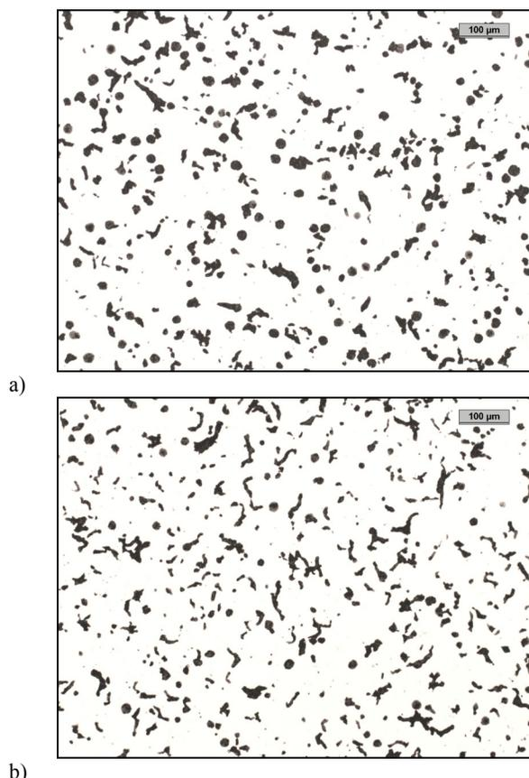
Fig. 1. Microstructure of castings with wall thickness of 5 mm:
