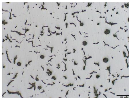
Wall thickness 16mm, 0.013%Mg, 15.2%SGI
