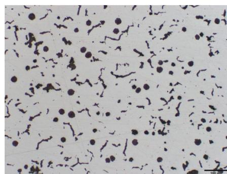
Wall thickness 8mm, 0.013%Mg, 24.9%SGI
