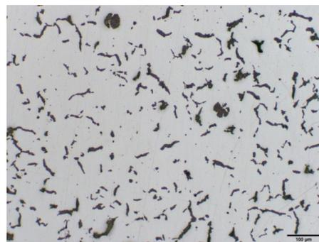
Wall thickness 40mm, 0.013%Mg, 1.5%SGI
