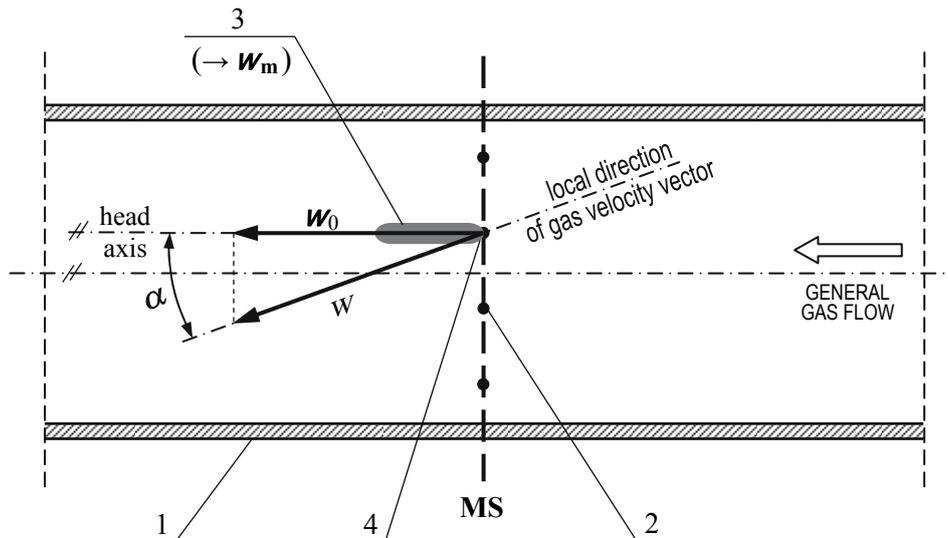
**Fig. 3.** Schematic illustration of the issue of accuracy of axial velocity measurement in situation of local gas flow deviation and setting the velocity sensor coaxially with the conduit, with gas velocity variation exclusively in plane parallel to conduit wall
