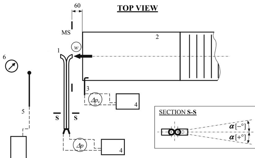
**Fig. 9.** System of measuring gas velocity with the S-type and L-type impact-pressure tubes under test
