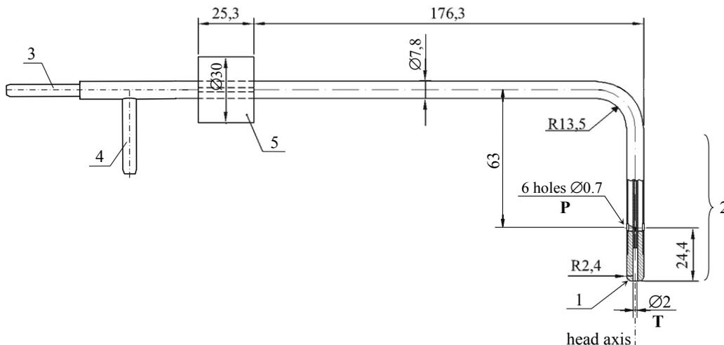
**Fig. 6.** L-type impact-pressure tube under test
