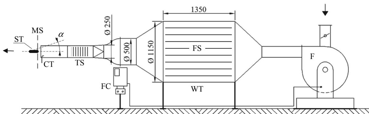
Fig. 7. General scheme of the test stand (in front view)
