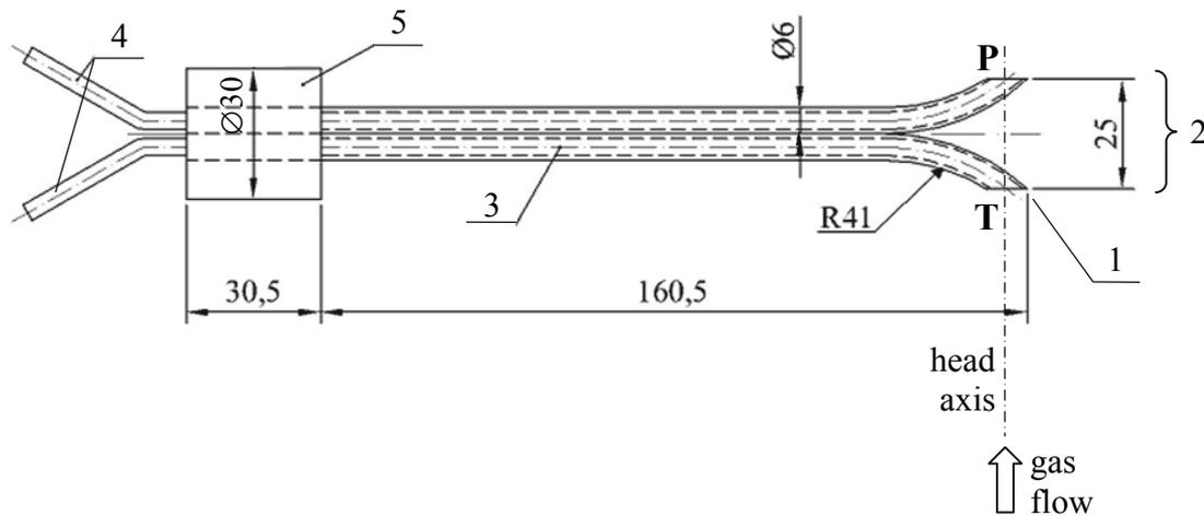
**Fig. 5.** S-type impact-pressure tube under test
