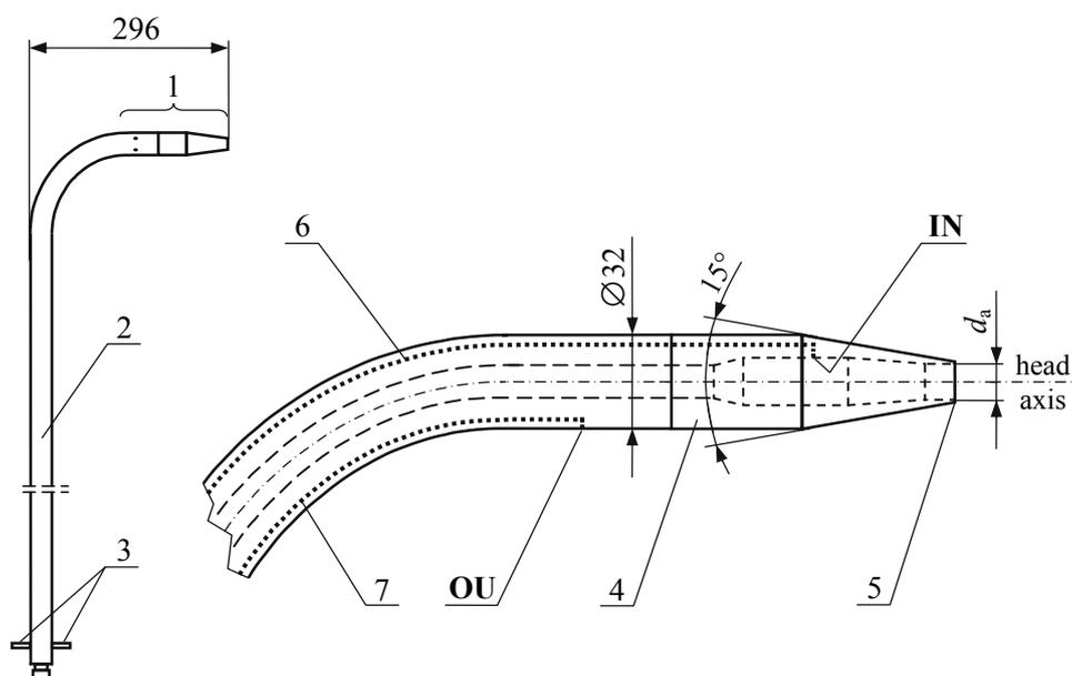
Fig. 4. Zero pressure probe under test
