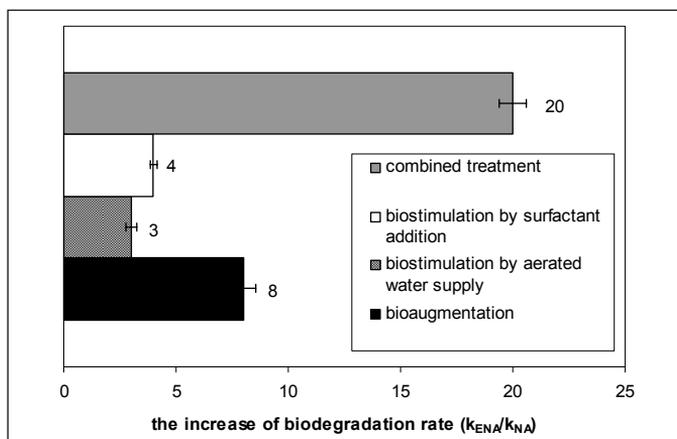
Fig. 5. The effect of enhancement methods on the biodegradation rate of oil hydrocarbons in soil
