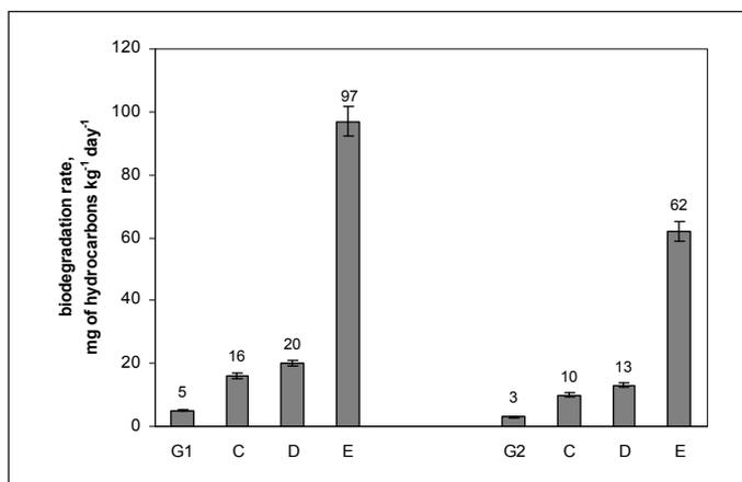
Fig. 4. The effect of biostimulation and combined treatment on biodegradation rates of oil hydrocarbons
