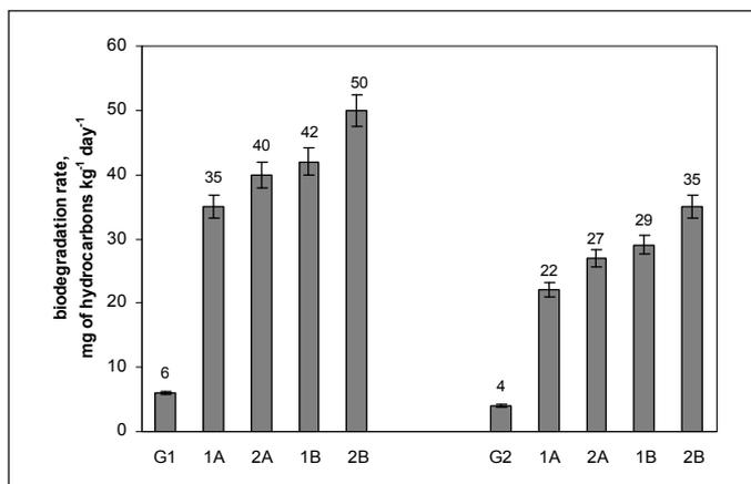
Fig. 3. The effect of bioaugmentation on biodegradation rates of oil hydrocarbons
