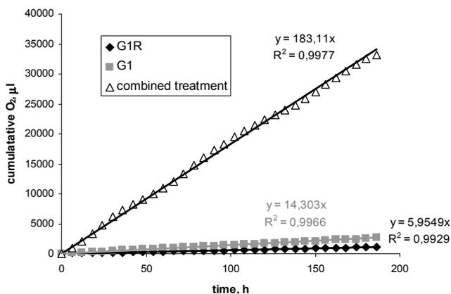
Fig. 2. The exemplary cumulative curves of O<sub>2</sub> uptake during intrinsic and enhanced biodegradation of oil hydrocarbons
