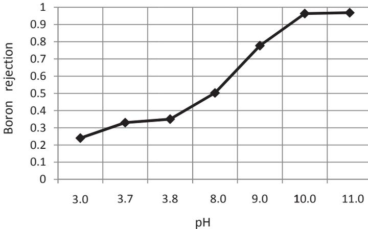
Figure. 4. Boron retention ratios as a function of feed pH
