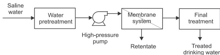
Figure 1. RO water desalination plant — simplified diagram [after 5,14]
