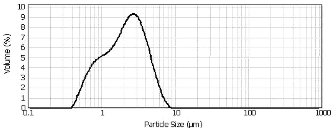
Fig. 1. Particle size distribution for calcium carbonate
