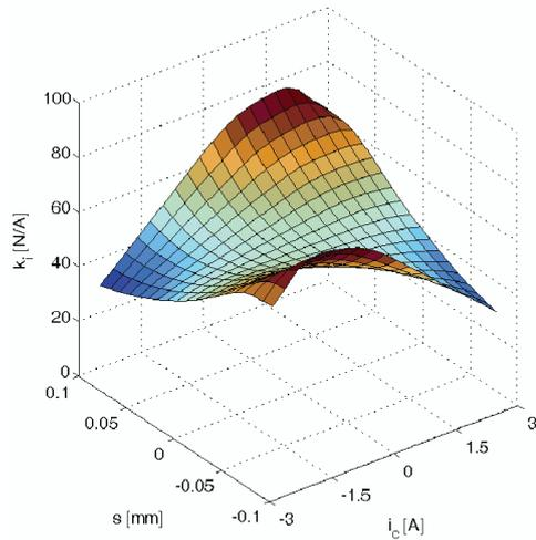
Fig. 4. Current gain value vs. the control current  $i_c$  and position of the rotor  $s$  for angle  $\beta_2 = 16^\circ$
