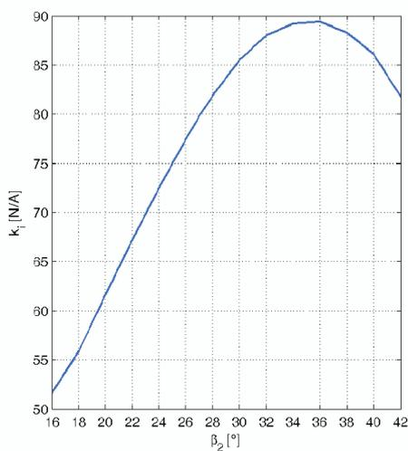
Fig. 6. Nominal current gain vs. the  $\beta_2$  angle
