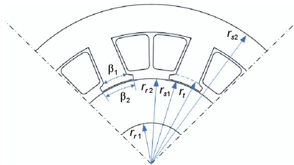
Fig. 3. Dimensions of the magnetic bearing actuator
