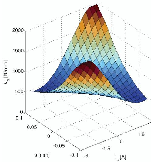
Fig. 5. Position stiffness value vs. the control current  $i_c$  and position of the rotor  $s$  for angle  $\beta_2 = 16^\circ$
