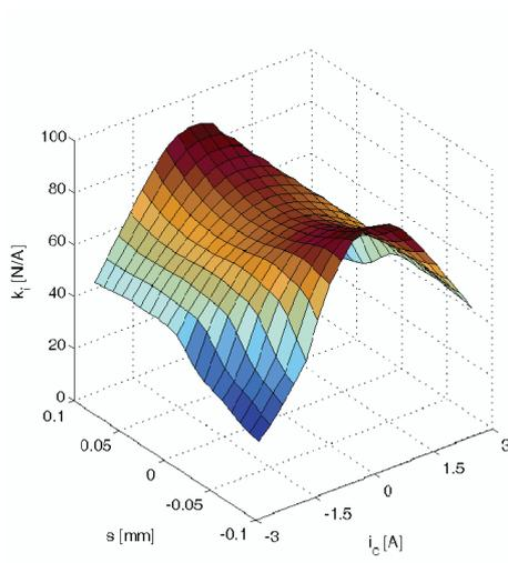
Fig. 9. Current gain vs. control current  $i_c$  and position of the rotor  $s$ , for  $\beta_2 = 25^\circ$
