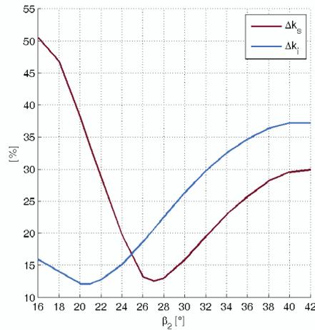
Fig. 8. The current gain and position stiffness variability vs. arc  $\beta_2$
