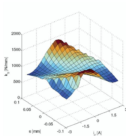
Fig. 10. Position stiffness vs. the control current  $i_c$  and position of the rotor  $s$ , for  $\beta_2 = 25^\circ$
