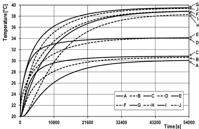
Fig. 2. Step response of the model of a floor heater in characteristic points
