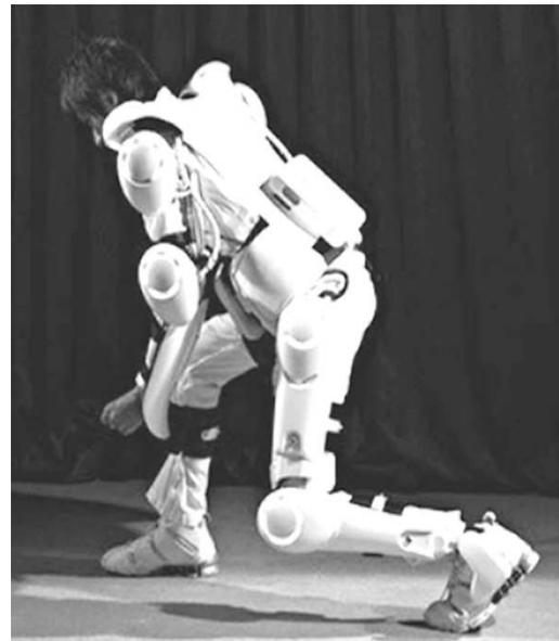
Fig. 7. HAL-5 exoskeleton [13]
