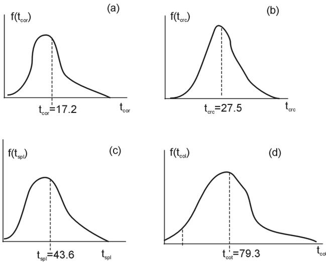
Fig. 4. Probability density functions of random variables  $t_i$  (years): (a) corrosion initiation time  $t_{cor}$ , (b) cracking initiation time  $t_{crc}$ , (c) spalling initiation time  $t_{spl}$ , (d) time to collapse  $t_{col}$
