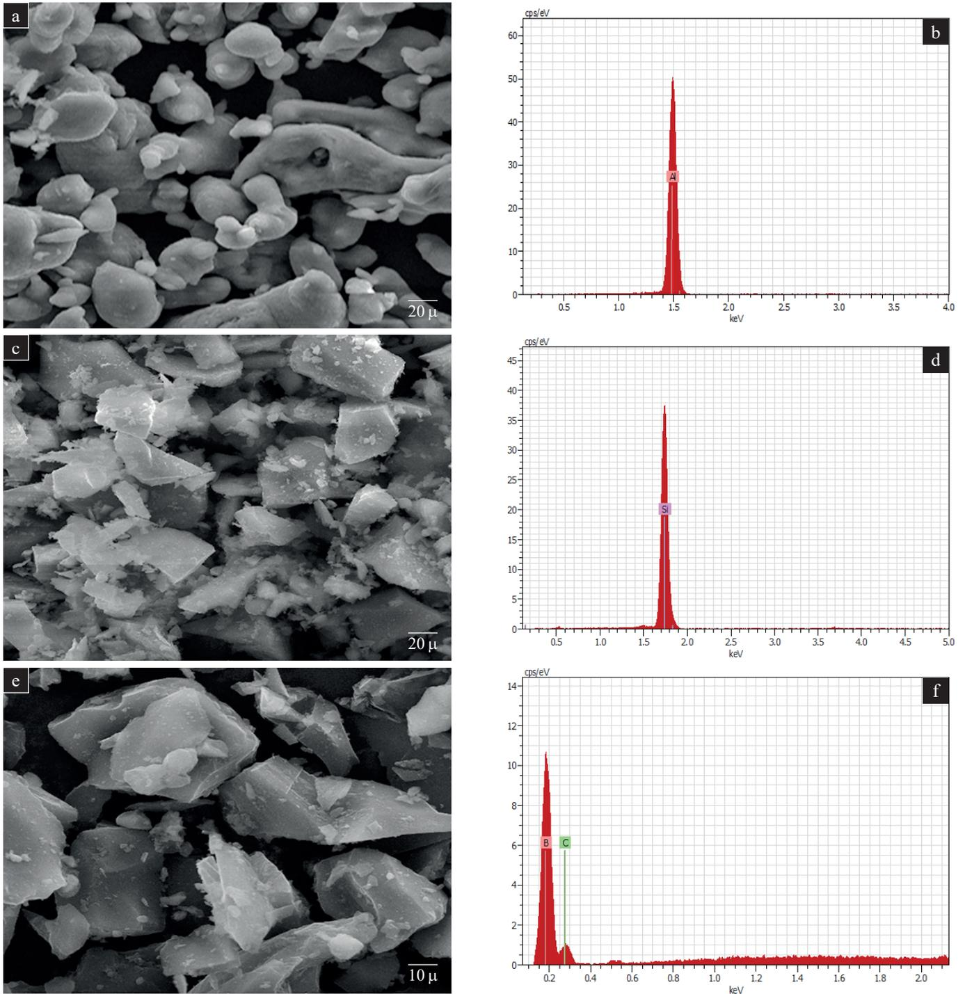
Fig. 1. Received powder SEM image (a) Al, (c) Si, and (e)  $\text{B}_4\text{C}$ , Also EDX analysis of (b) Al, (d) Si, and (f)  $\text{B}_4\text{C}$
