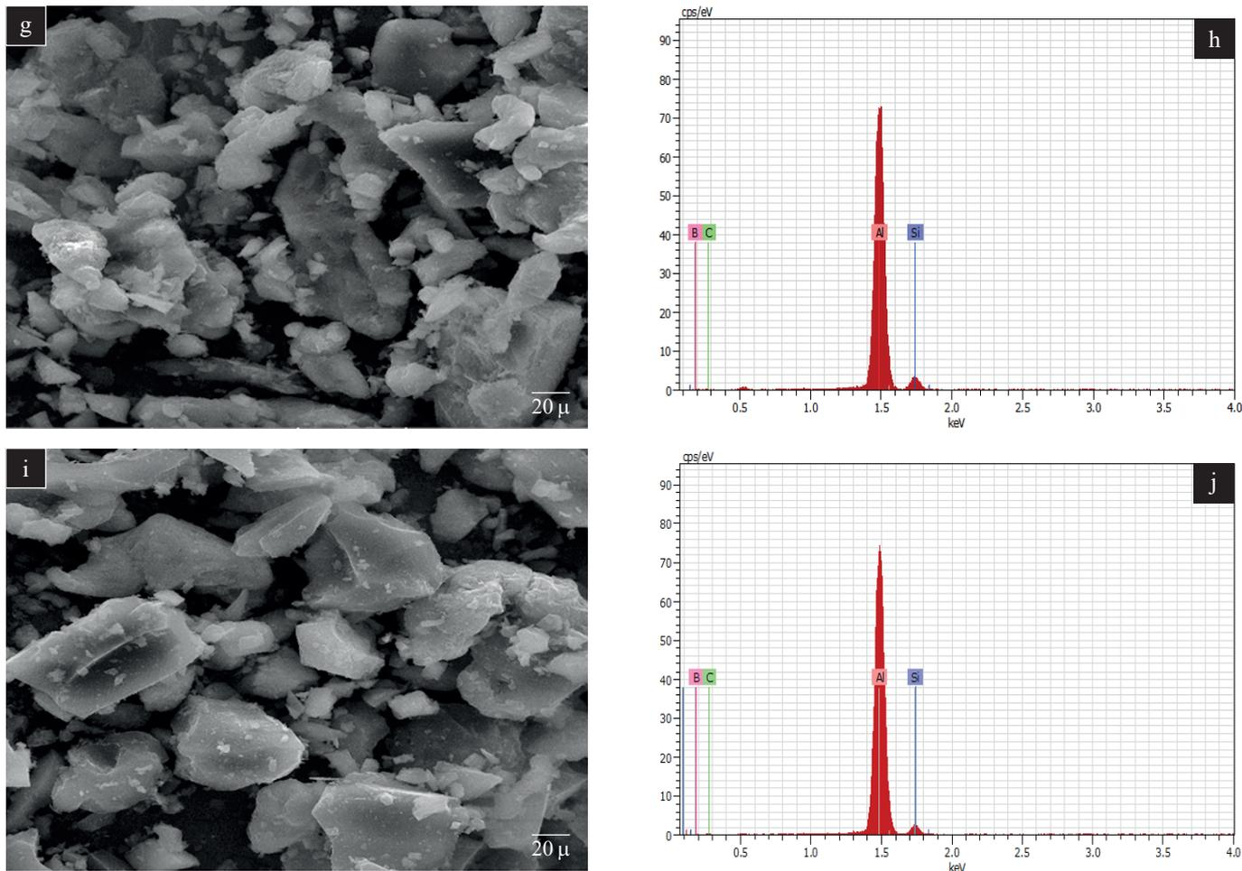
Fig. 2. Mixed powders SEM and EDX analysis of: g-h) Al-Si-8B<sub>4</sub>C, and i-j) Al-Si-10B<sub>4</sub>C composites
