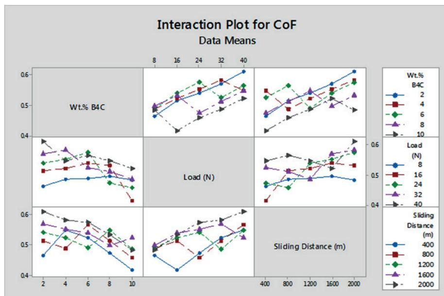
Fig. 4 The interaction plot for CoF vs wt.%B<sub>4</sub>C, load, sliding distance
