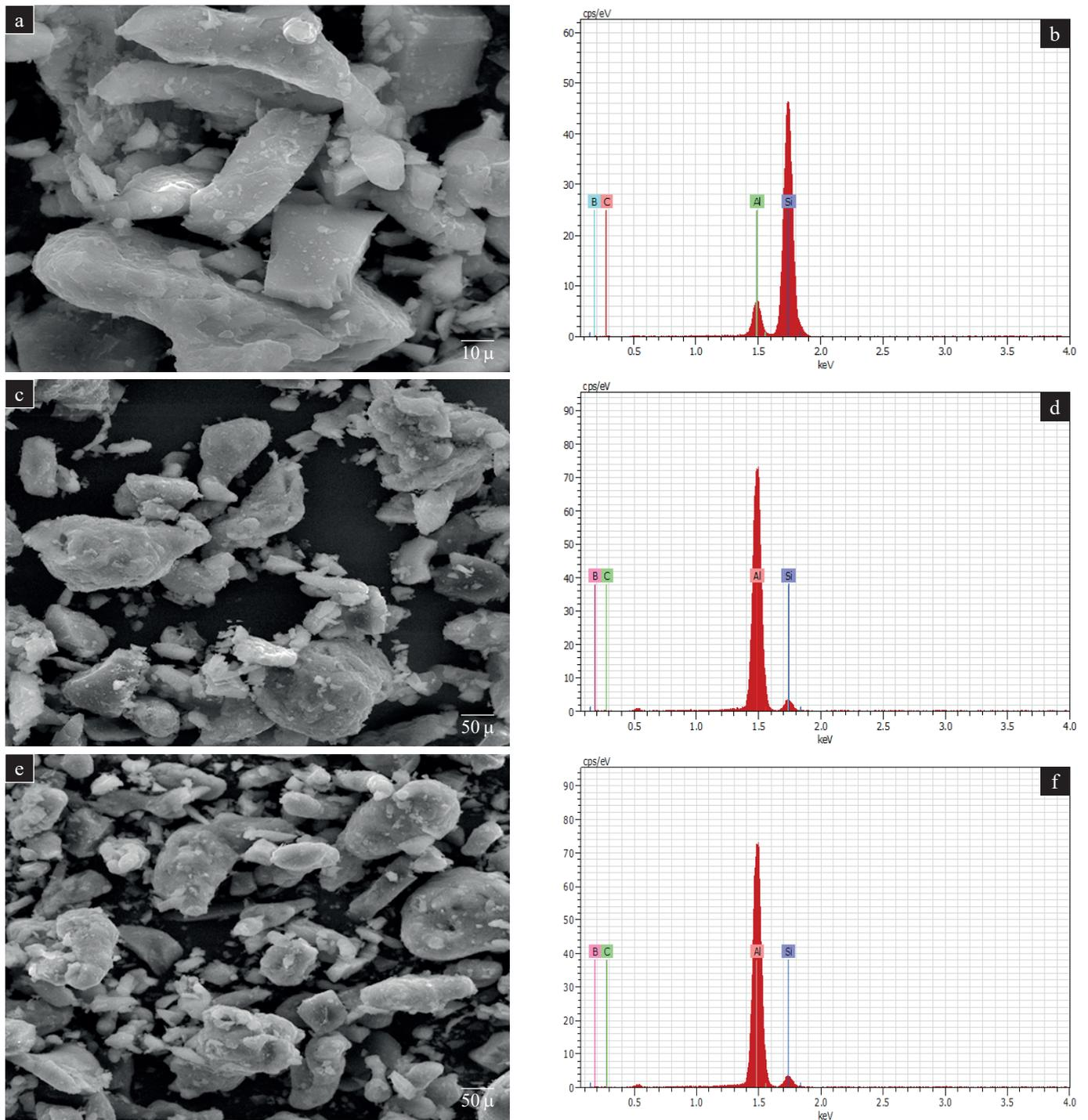
Fig. 2. Mixed powders SEM and EDX analysis of: a-b) Al-Si- $2B_4C$ , c-d) Al-Si- $4B_4C$ , e-f) Al-Si- $6B_4C$  (continued on next page)
