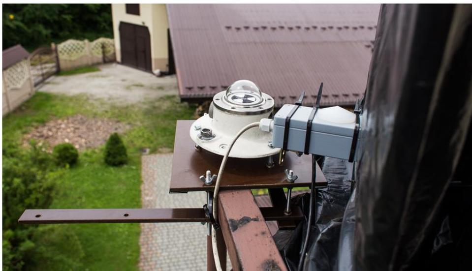
Fig. 3. Eppley solar radiation density meter
