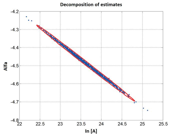
Fig. 8. Characteristic parameter values obtained in 1000 simulations of experiment and approximation – points, and confidence ellipse – solid line
