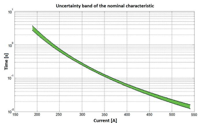
Fig. 9. Uncertainty band of the current-time characteristic calculated on the basis of the confidence ellipse, with the dark lines marking the boundary characteristics according to the further specified confidence interval of operation time
