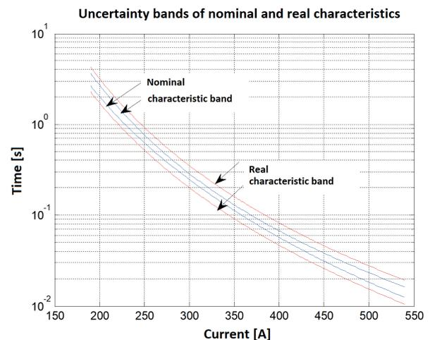
Fig. 10. Uncertainty bands of nominal and real current-time characteristics
