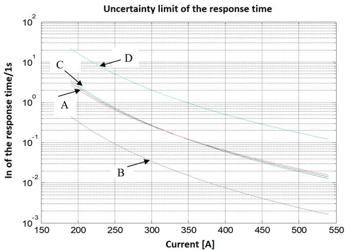
Fig. 7. Limits of uncertainty current-time characteristic of the tested fuses determined on the basis of confidence intervals of approximation parameters: A:  $A_n, \max_{n, \min}$ ; B:  $A_n, \min_{n, \min}$ ; C:  $A_n, \min_{n, \max}$ ; D:  $A_n, \max_{n, \max}$
