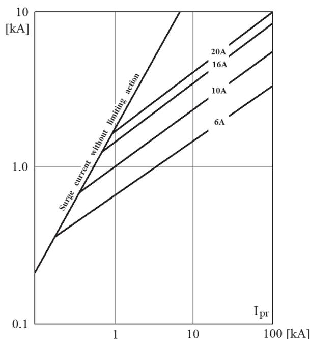
Fig. 1. Characteristic of limiting current for fuses
