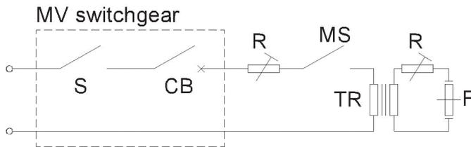
Fig. 3. Laboratory setup for testing MV fuses located at the Short Circuit Laboratory of the Institute of Electrical Power Engineering
