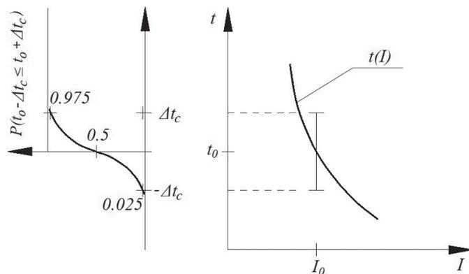
Fig. 2. Time-current characteristic of a fuse and its statistical description of uncertainty for assumed confidence level of 0.95
