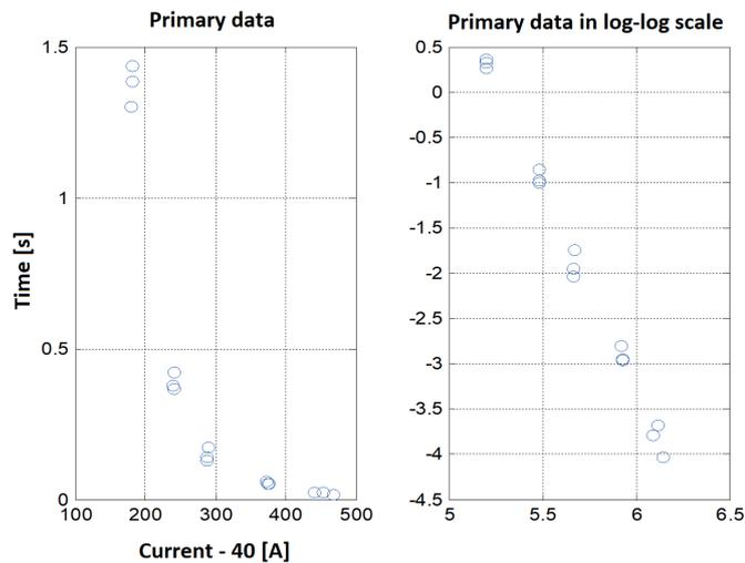
Fig. 4. Primary data – results of measurements of operating time of 15 fuses with rated current of 40 A
