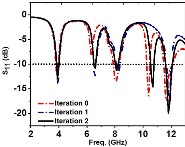
Fig. 3.  $S_{11}$  Evolution plot of the proposed antenna
