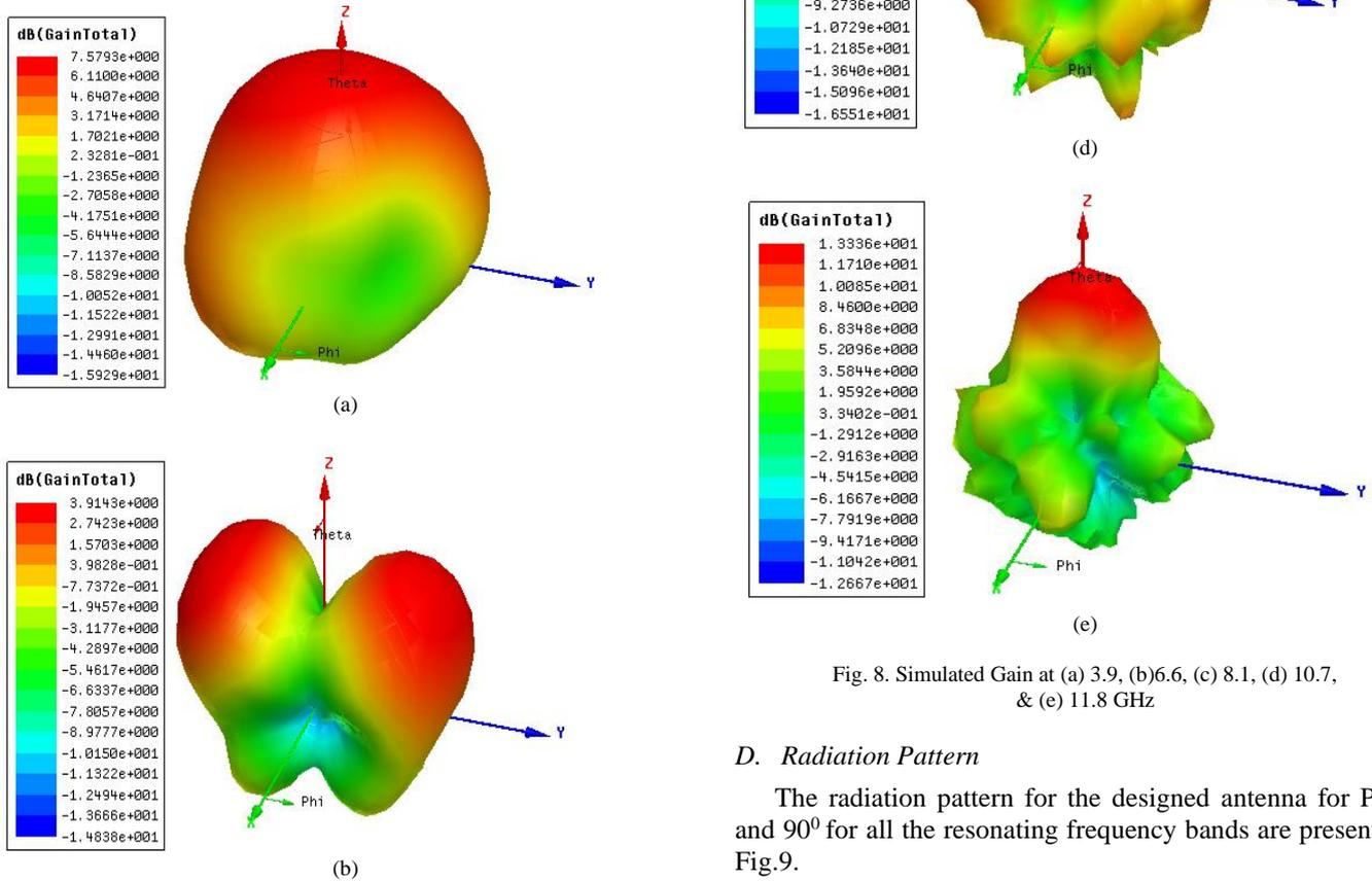
Fig. 8. Simulated Gain at (a) 3.9, (b)6.6, (c) 8.1, (d) 10.7, & (e) 11.8 GHz
