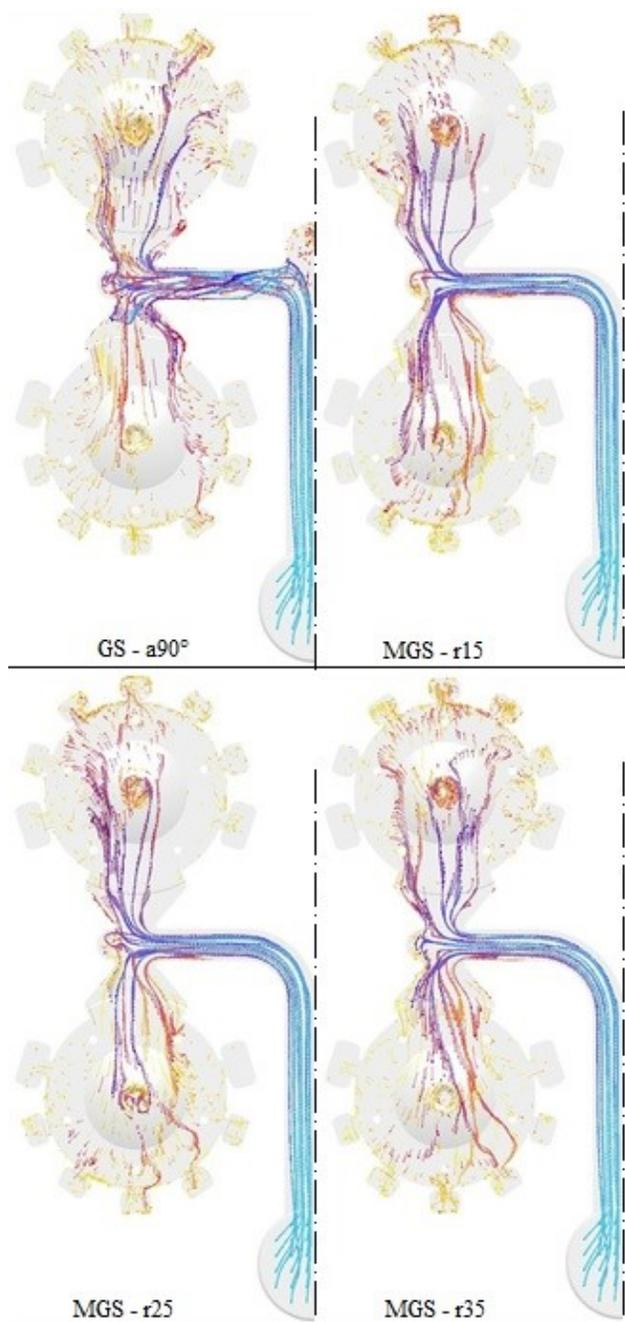
Fig. 3. Melt flow in runners
