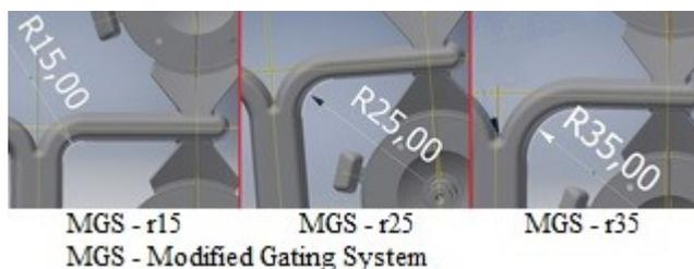
Fig. 2. Modified main runner branching solutions
