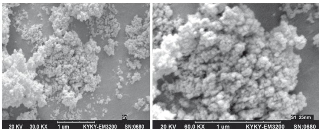
Fig. 1. Scanning Electron Microscopy (SEM) images of synthesized silica nanoparticles in different zoom
