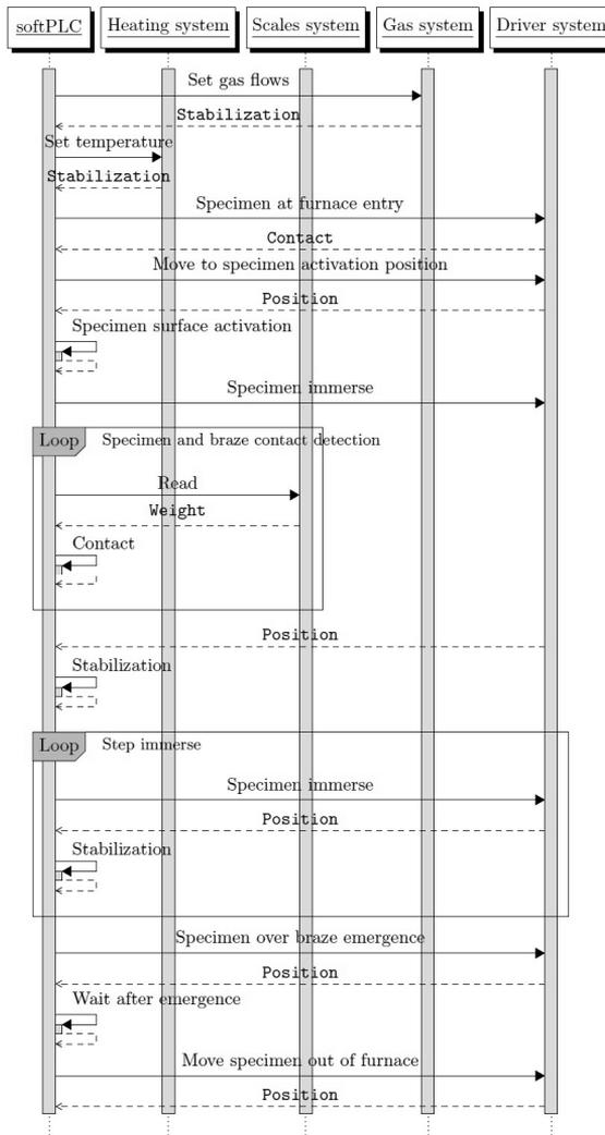
Fig. 5. A flow diagram of the measurement experiment.
