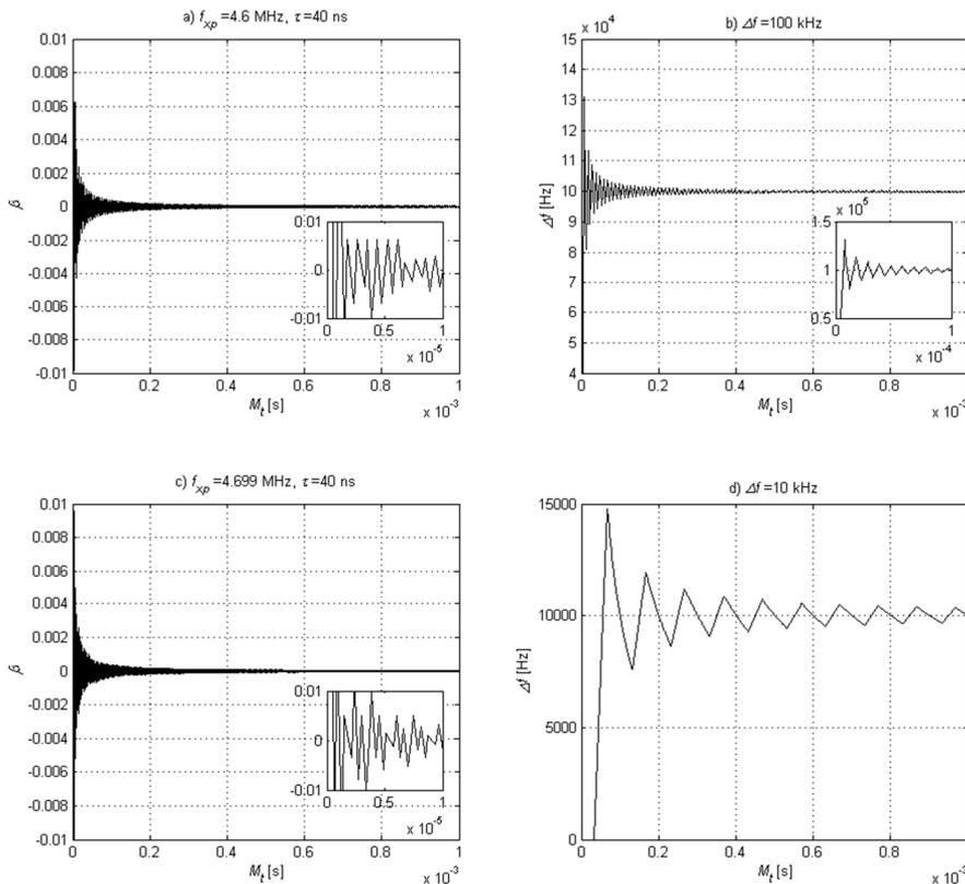
Fig. 5. The relative error in the frequency measurement process for  $f_{xp} = 4.6$  MHz (a);  $f_{xp} = 4.699$  MHz (c). Measurement of the frequency shift  $\Delta f = 100$  kHz (b);  $\Delta f = 10$  kHz (d).
